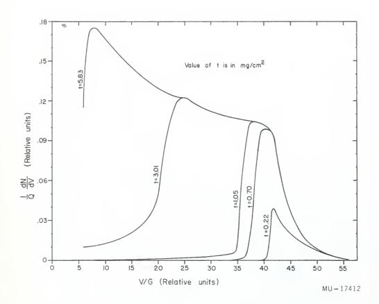
Fig. 2. Computed differential pulse-height spectra for different thicknesses of bismuth.  $Q = \phi \sigma n A$ , and (R - r) assumed to be 9.2 mg/cm<sup>2</sup>.
